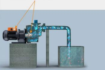
The self-priming pumps is equipped with a microelectronic protector, using intelligent microelectronic real-time online monitoring technology, when the pump is phase loss, to achieve Fast circuit breaking protection.
