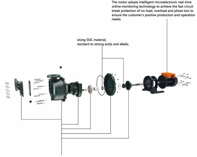
The pump head materials are PP and PVDF, which adapt to different liquids working conditions.
