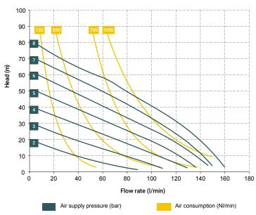
\* The curves and performances refer to pumps with immersed suction and open delivery outlet with water at 20 °C and vary according to the composition materials.
