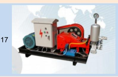
Model: GPB-150/11 Pressure: 8 MPa Displacement: 6-9/h<sup>3</sup> Motor power: 11 kW
