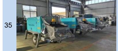
Model: 90D hydraulic wet spraying machine Required air compressor configuration: 90 kW 16 cubic meters or more Displacement: 4-6/h Motor power: 22 kW Horizontal maximum distance is about 90 meters
