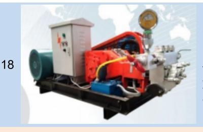
Model: XPB-10/22 Pressure: 15 MPa Displacement: 6-9/h<sup>3</sup> Motor power: 22 kW
