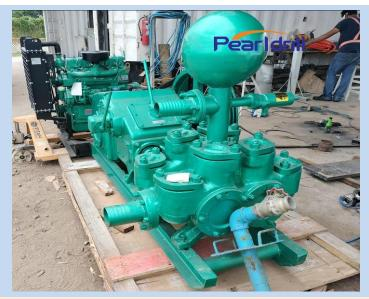
BW850/2 mud pump Cylinder diameter:150 mm Piston Stroke:180 mm
