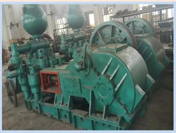
BW1100 mud pump Piston stroke (mm): 240
