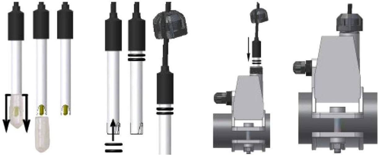
**Fig. 3 – Mounting the probe in the probe-holder**
